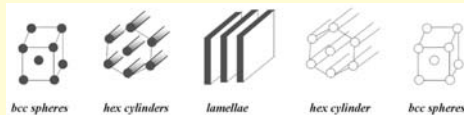
Figure 1: Common microphase separated structures observed in block copolymers (e.g., SB diblock copolymer, dark component as polybutadiene).
